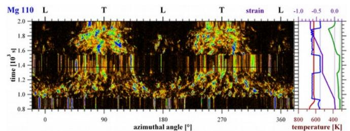
**Figure 5:** Materials-Oscilloscope plot of magnesium undergoing high-temperature plastic deformation.<sup>5</sup>
