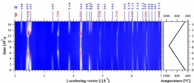
**Figure 4:** Study of defect kinetics by the decrease of intensity due to extinction, described by the dynamical theory of diffraction: Time evolution of diffractograms from Zr-2.5Nb undergoing a heating-cooling cycle.<sup>6</sup>
