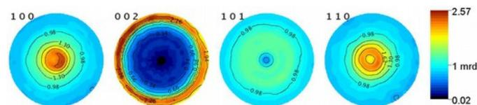
**Figure 3:** Texture study of magnesium showing the basal plane normals oriented perpendicular to the extrusion axis.<sup>4,5</sup>
