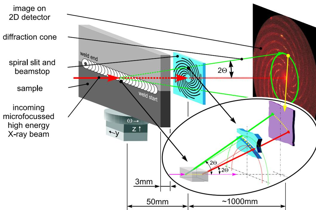
Figure 6.7.3: Schematic of setup with spiral slit system for non-destructive depth resolved phase and strain investigations. The inset visualizes the principle of the beam path which leads to the spatial resolution.
