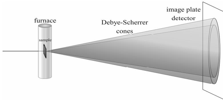
**Figure 1:** Diffraction setup with high-energy X-rays around 100 keV in transmission for in-situ experiments. The polycrystalline sample is located in a furnace, performing powder-diffraction in the monochromatic beam which arrives from the left. Debye Scherrer rings can be recorded in the far distance.
