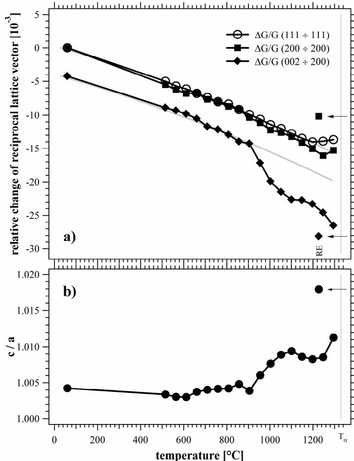
**Figure 7:** Temperature dependence of (a) reciprocal lattice vectors and (b)  $c/a$  ratio of the  $\gamma$ -phase. The arrows mark the data points RE, see Figure (3), after re-entering the  $\gamma + \alpha$ -phase field from above  $T_{\alpha}$ .
