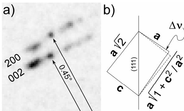
**Figure 5:** Correlated reflections on the  $\gamma$ -200 /  $\gamma$ -002 ring pair (a) which stem from a domain boundary (b).
