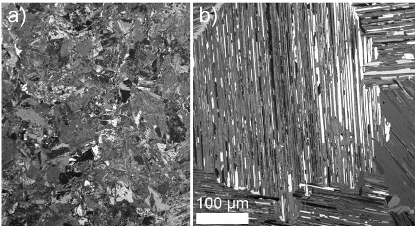
**Figure 2:** Microstructure of the sample before a) and after b) the heating cycle as shown in Figure (3). The massively transformed starting material recrystallizes into a fully lamellar structure.
