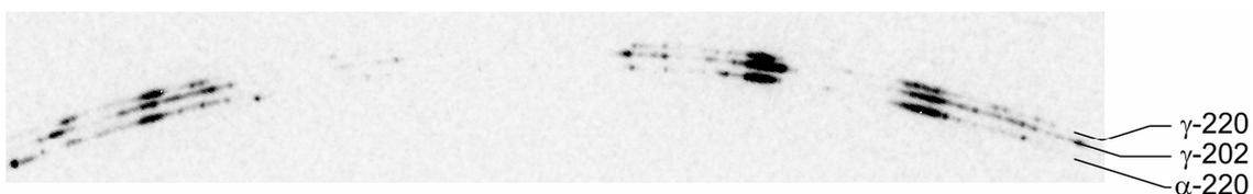
**Figure 6:** Correlated reflections on the  $\gamma$ -220,  $\gamma$ -202,  $\alpha$ -220 ring triplet proofing the Blackburn relation between the two phases.
