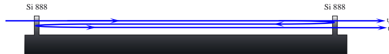
Figure (3): Sketch of the cavity with the two active slices sticking out of the monolithic device within a distance of 150 mm. Photons impinging from the left can be trapped due to transmission and reflection probabilities T and R , respectively. They exit the cavity with probabilities TT , TRRT , TRRRRT \dots T^2R^{2N} for 0, 1, 2 \dots N back and forth bounces, being delayed by N times the time of flight inside the cavity of 1.0 ns. The reflection angle is adjusted to exactly 180 degree and the beam paths of multiply reflected photons are truly superimposed in space.
