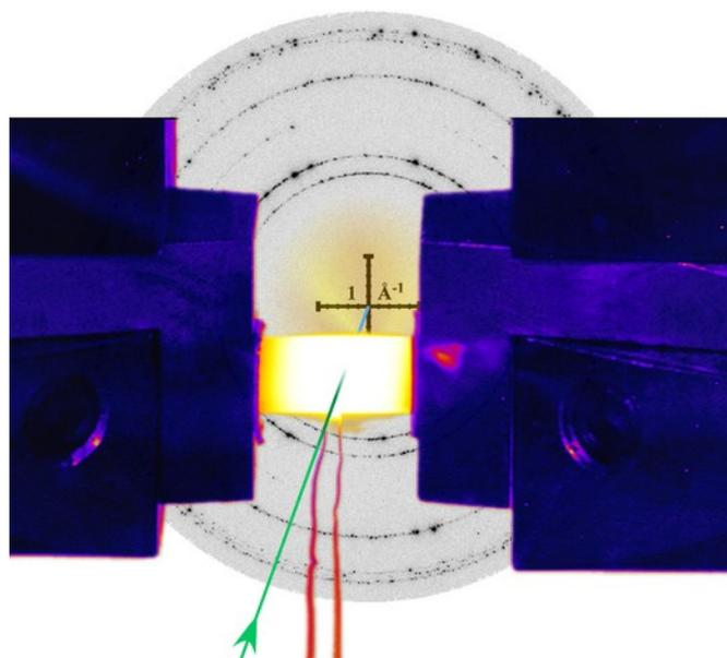
**Figure 1:** The Materials Oscilloscope – in-situ diffraction measurement of a glowing sample, being compressed (foreground) while time-resolved, two-dimensional diffraction patterns are taken (background).<sup>1,2</sup>
