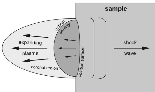
FIG. 9. Schematic view of shock wave generation as a result of laser impact.
