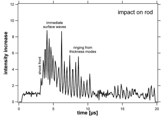
FIG. 6. Intensity normalized to unity for the undisturbed crystal as a function of time measured on the tensile strain side while impacted on the rod side. Ringing of the thickness modes is seen immediately after the arrival of the shock front.
