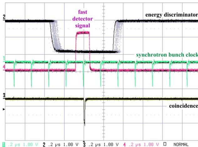
FIG. 3. (Color online) Coincidence of the different detector and synchrotron bunch clock pulses for the timing setup.
