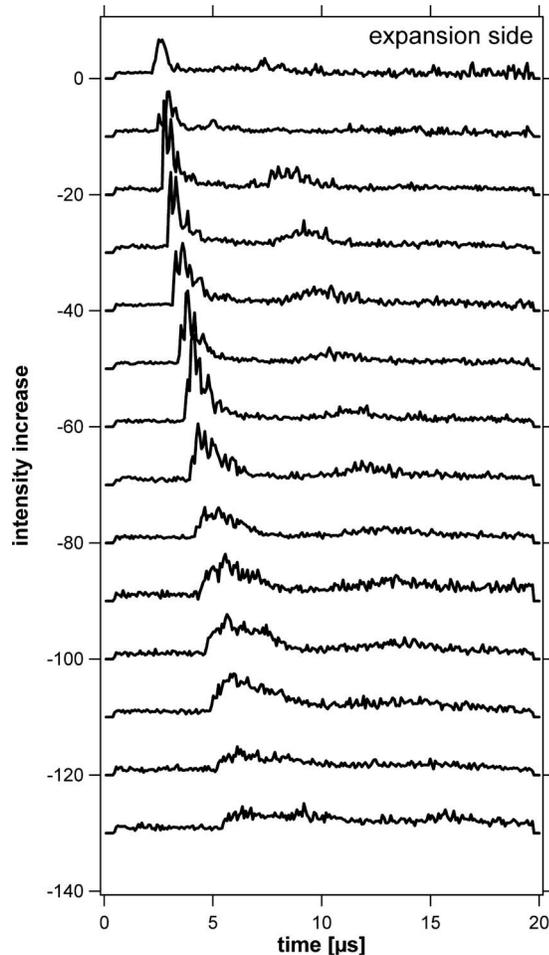
FIG. 8. Time dependent intensity profiles as in Fig. 6 as a function of position in the rod. The curves were recorded at intervals of 2.5 mm along the rod. The top curve is close to the impact surface.
