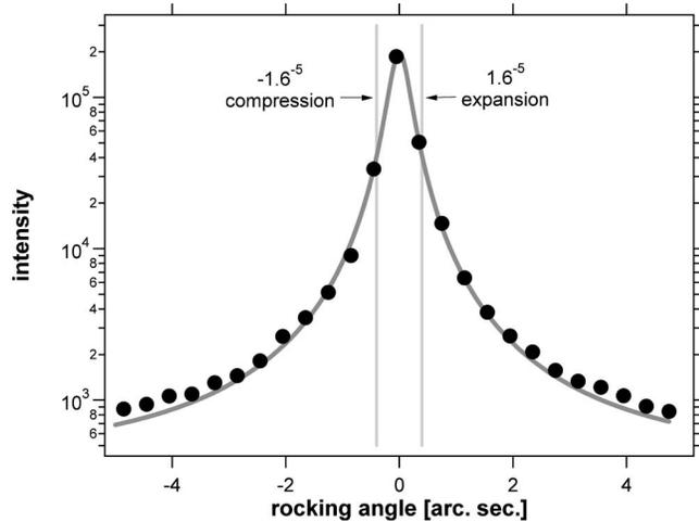
FIG. 4. Rocking curve of the Si 333 reflection of the sample against the monochromator showing an ideal Lorentzian shape and line width. The compressive and tensile strain positions where the time-resolved signals were collected are shown.
