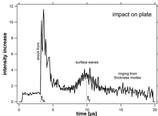
FIG. 5. Intensity normalized to unity for the undisturbed crystal as a function of time measured on the tensile strain side while impacted on the plate side. Arrivals of the shock front  $t_s$  and of the broad pulse distribution  $t_r$  are indicated.
