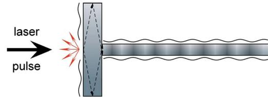
FIG. 10. (Color online) Suggested path for ultrasonic waves resulting from laser impact on the plate. Some longitudinal waves travel inside the plate along the dotted path and combine in a compressive way to produce thickness variations coupled to surface waves in the rod.
