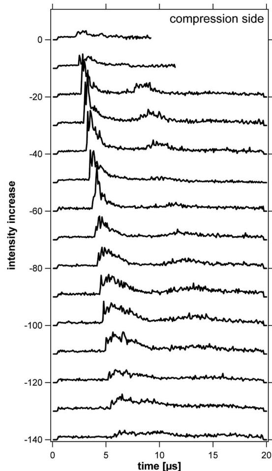
FIG. 7. Time dependent intensity profiles as in Fig. 5 as a function of position in the rod. The curves were recorded at intervals of 2.5 mm along the rod. The top curve is close to the impact surface.
