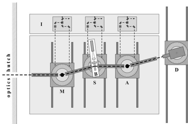
FIG. 1. General layout of the triple crystal diffractometer with monochromator (M), optional analyzer (A), detector (D), and interferometric angle encoders (I). The whole laser and sample system has been mounted onto an optical bench (B) on top of the sample stage (S).
