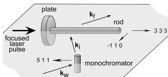
FIG. 2. Double crystal setup between monochromator and rod-plate shaped sample indicating the crystallographic directions and the x-ray and laser beams.
