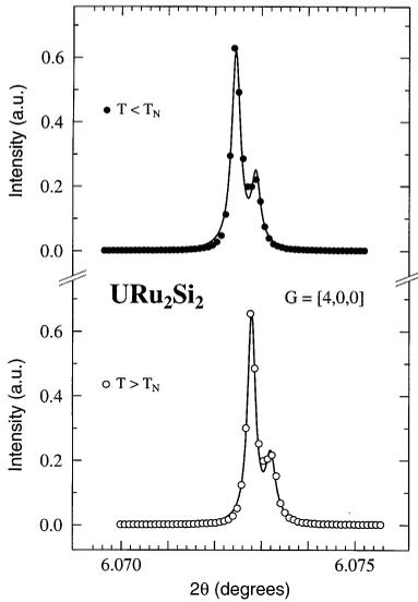
Fig. 1. X-ray intensity as a function of the scattering angle  $2\theta$  recorded for the scattering vector  $G = [4,0,0]$ . The upper and lower panels present the pattern recorded below (at 14.38 K) and above (20.22 K) the Néel temperature, respectively. The solid line in each panel is a fit with the sum of two Lorentzian functions. These results show that  $\text{URu}_2\text{Si}_2$  remains tetragonal in the ordered state.
