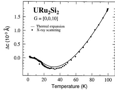
Fig. 2. Thermal variation of the lattice parameter  $c$  of  $\text{URu}_2\text{Si}_2$  as measured in this work by high-energy X-ray diffraction (points) and deduced from the thermal-expansion measurements of Kuwahara et al. (solid line) [9].
